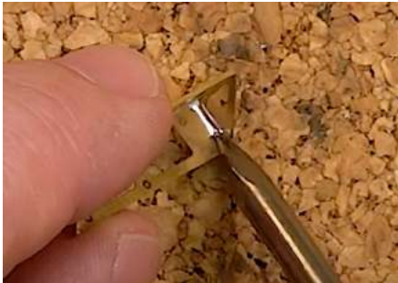
Fig. 16. Soldering photoetch parts. (FineScale Modeler)
