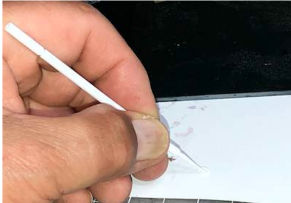
Fig. 23. Picking up a bit of tacky glue on a disposable paint brush.
