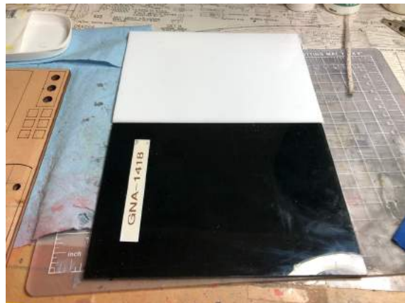
Fig. 20. Black and White glass pieces used for cutting and manipulating PE.
