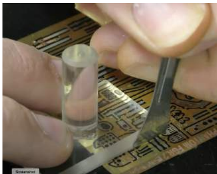
Fig. 13. Photoetch cut off tool for cutting such parts (Genessis-Models.co.uk)
