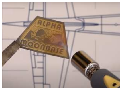
Fig. 15. Heating a piece of photoetch to soften it for easier bending and shaping. (FineScale Modeler)
