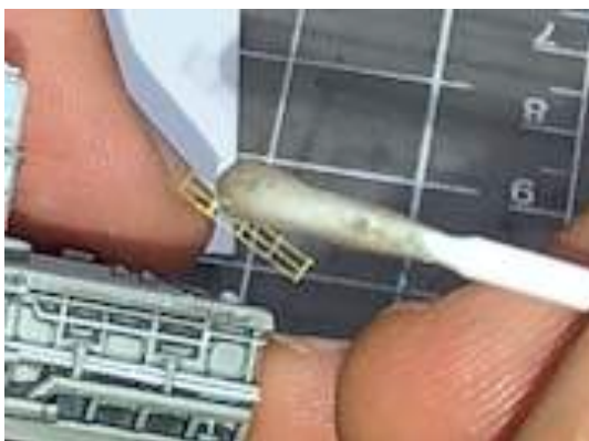
Fig. 25. Picking up a PE rail with a Pic-n-Stic .
