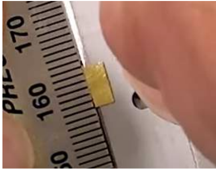
Fig. 14. Bending photoetch with a razor blade against a steel ruler. (FineScale Modeler)
