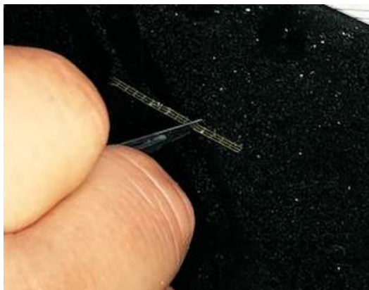
Fig. 21. Cutting PE with a scalpel on black glass.
