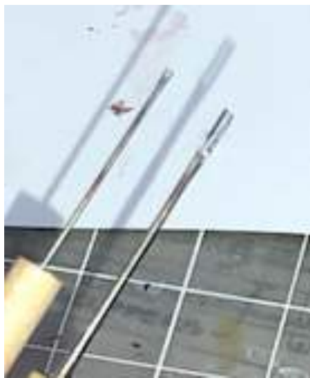
Fig. 27. CA glue applicators made from half clipping the eyes of sewing needles.
