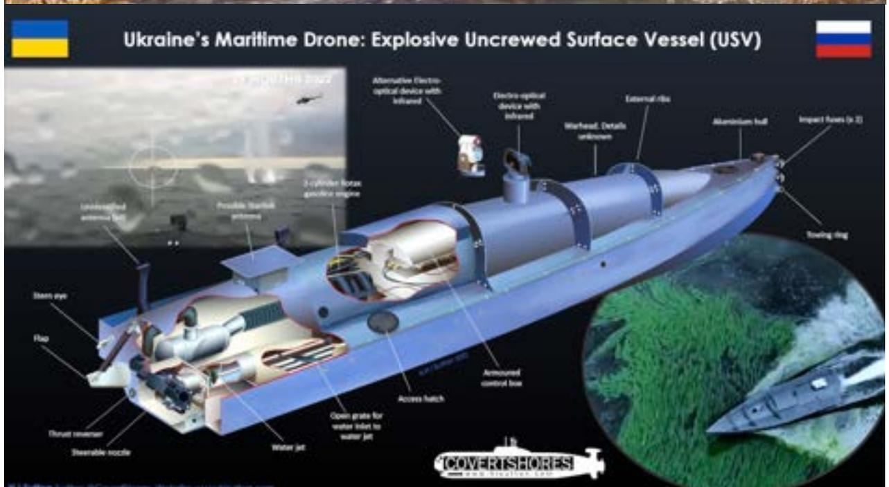
Fig. 6. (above) A Ukrainian USV washed up on shore outside the entrance to Sevastopol harbor. (below) Schematic of one of these USVs (H.I. Sutton).
