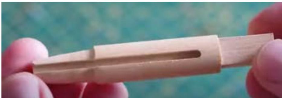
Fig. 15. Jig for making rope hanks (Carlo, [Tagliamare](#))
