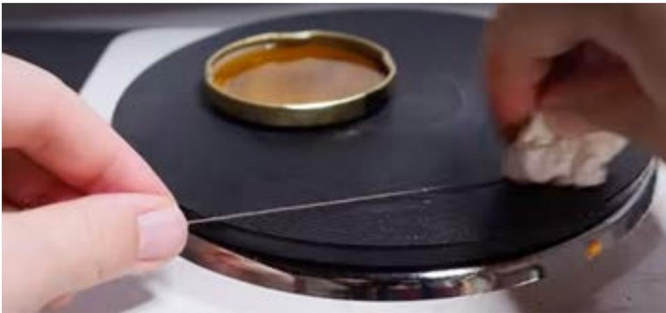
Fig. 14. Treating rigging line with melted beeswax. (Carlo, [Tagliamare](#))
