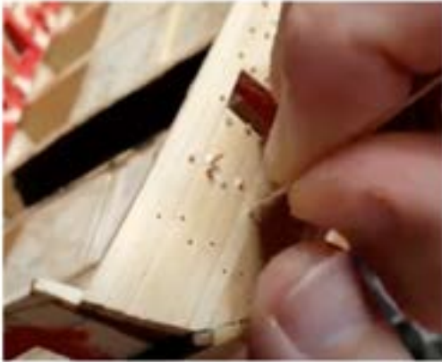
Fig. 15. From a video on how to apply scale treenails to a model ship ( Modelship Builder ).
