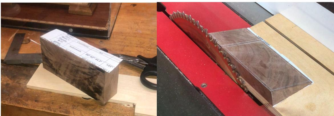
Fig. 8. **Left**-gluing piece of paper onto surface of small subject wood piece. **Right**-then gluing the small subject wood piece to a larger piece of  $\frac{1}{2}$ " plywood with the paper sandwiched in the glue joint and making the needed cut with your hands safely away from the saw blade.
