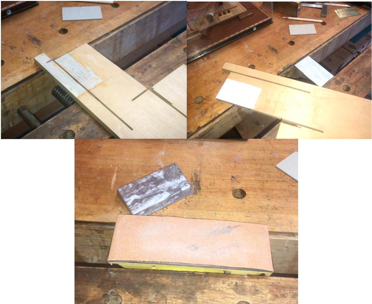
Fig.10. **Upper left**-the subject piece of walnut is clamped to a vise under the plywood. **Upper right**-the scrap plywood is pulled off the subject piece in the vise with the separation going through the paper. **Bottom**-the left-over paper is sanded off the subject piece.
