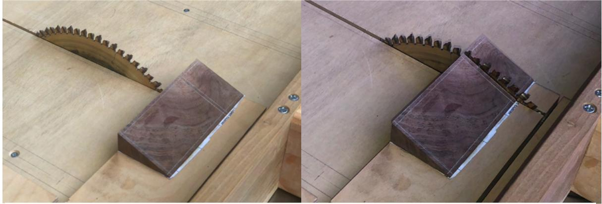
Fig.9. Cross-cuts can also be made in this way as well. It is done here on a cross-cut sled.
