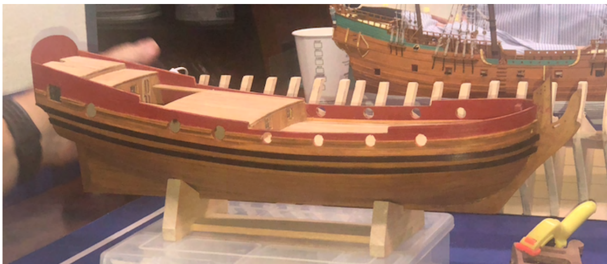
Fig. 16. The planking and wales of Clare Hess's Charles Royal Yacht are now completed!
