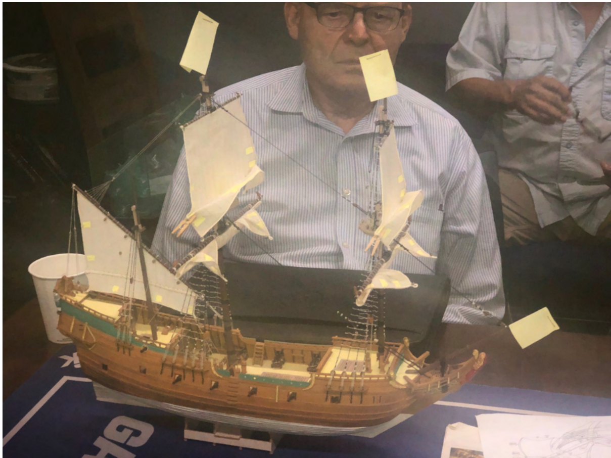
Fig. 15. George Sloup installing the sails on his Papegojan model. Note the furling courses on the fore and main masts.
