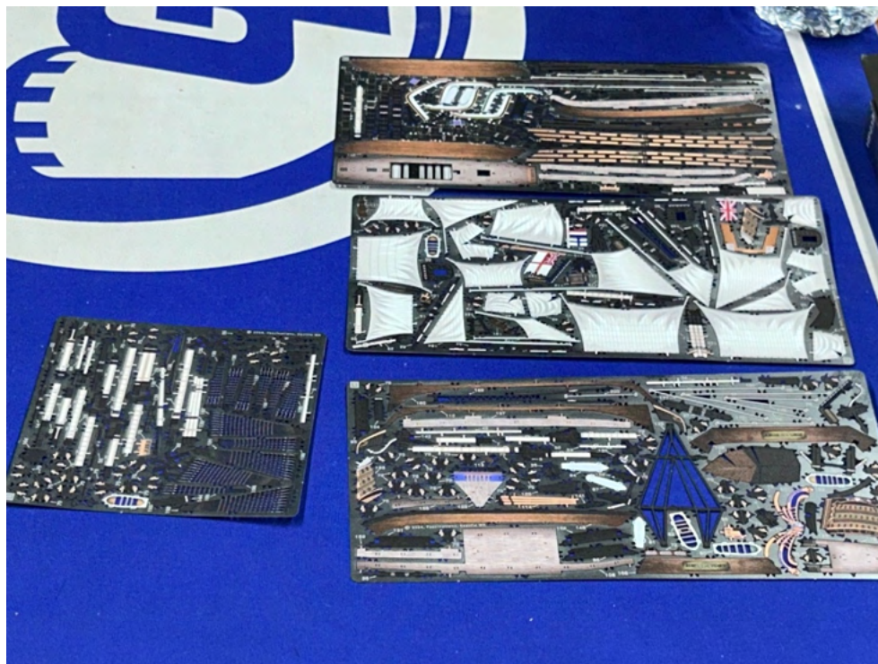
Fig. 10. Parts from an HMS Victory model done in photoetched metal by Metal Earth Models brought by John Garis. Fascinating how many of the parts have color anodized onto the metal.
