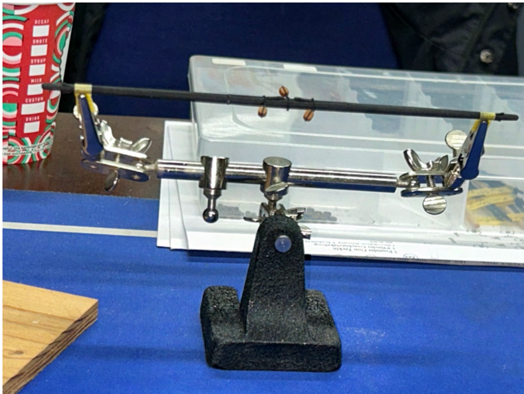
Fig. 22. Setup for rigging one of the yards.
