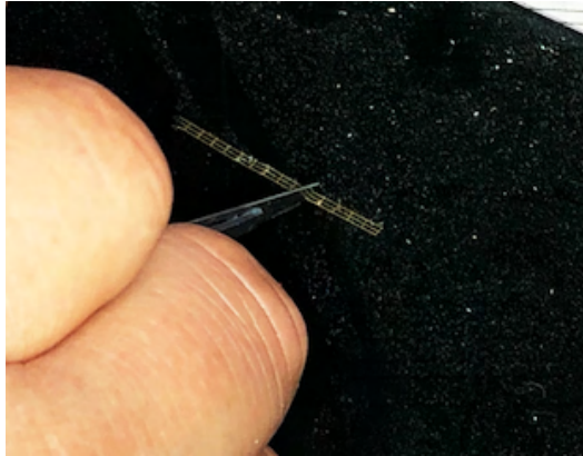
Fig. 9. Cutting PE with a scalpel on black glass.
