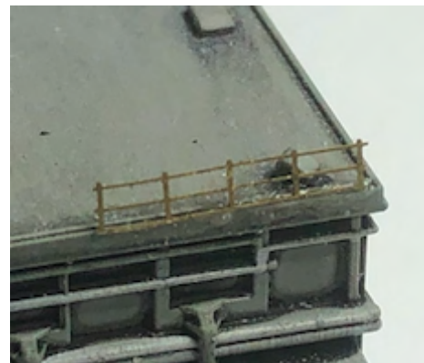
Fig. 14. Precise placement of the PE rail where it belongs sticking via tacky glue.
