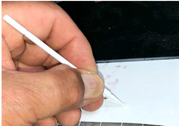
Fig. 11. Picking up a bit of tacky glue on a disposable paint brush.
