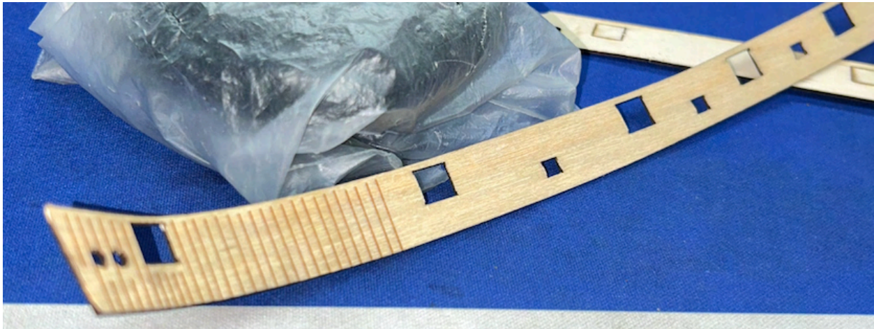
Fig. 9. Kerf bending a plank. The demo, I believe, courtesy of Clare Hess.
