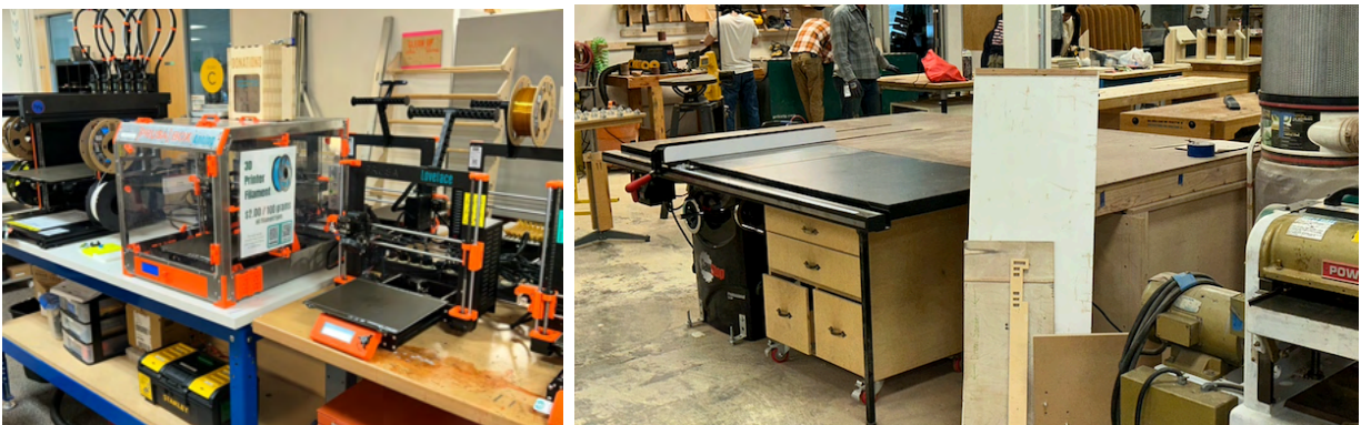
Fig.10. Left-3D printer. One of several. Right- SawStop brand table saw with a generous outfeed table.
