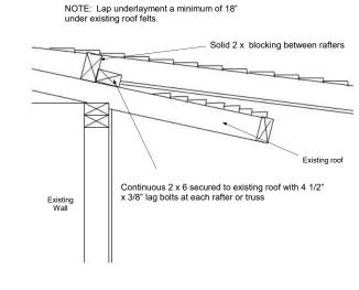
Detail A Sample attachment details Detail B
