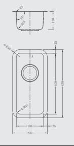
■ Undermount bowl ■ Satin finish ■ Insusound<sup>®</sup> 🖗 ■ 3½" basket strainer waste and concealed overflow included ■ Maximiser plumbing kit included ■ Individually boxed ■ Steel thickness 1.2mm ■ Cut out template
