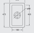
PLEASE NOTE: A DXF is not available, sink should be used as template. When undermounting, a minimum gap of 4mm must be left between the sink and the worktop.
