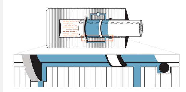
The core of the patented NextSeal technology is to balance the gas pressure with an equal liquid pressure on the other side of the seal
