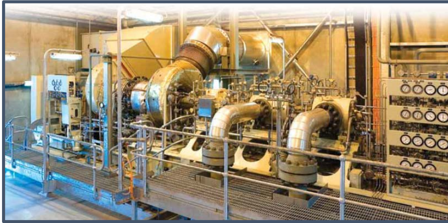
Solar GT driven tandem, skid mounted
