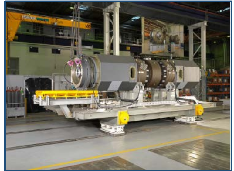
MAN HS electric motor driven tandem unit
