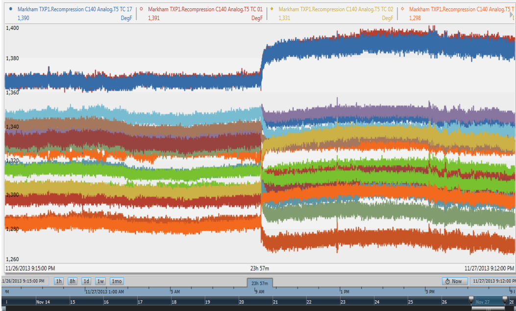
T5 temperature plot as it is shown in a Pi Vision trend. This actual graph of a step change in a Turbine temperature spread associated with further degradation of the insulation.
