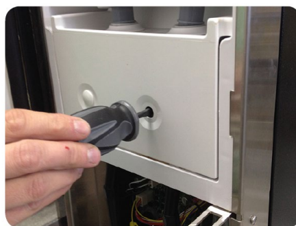
Adjusting Water Flow Using Flat Blade Screwdriver
