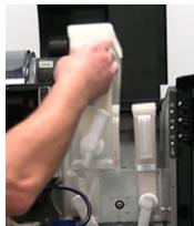
Using the handle, lift up and slide each canister out and put them on a flat, clean surface.
