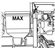
*Do not overfill the coffee canister.*
