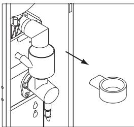
2. Remove the steam collector by pulling it forward and twisting in a clockwise rotation.
