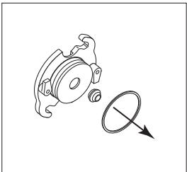
7. Slip the O-ring off the Whipper Chamber Receptacle and remove the shaft seal.
