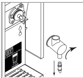
4. Twist the Whipper Chamber clockwise and pull it off the Whipper Chamber Receptacle.
