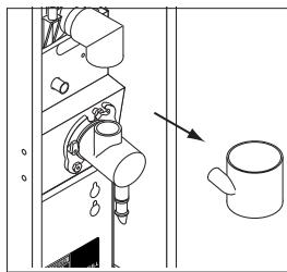
3. Pull the Mixing Chamber out of the Whipper Chamber.
