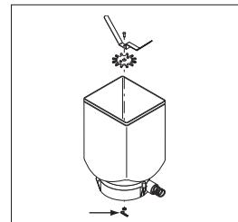
4. Remove the Wiper Blade and Drive Gear by removing the Retaining Clip from the Wiper Blade Shaft.
