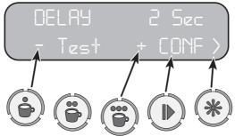
What is the **single impulse**: immediately after having any dosage of coffee, the machine will always place itself in the "single impulse" mode for a brief period of time (the  $\bigcirc$  button will flash), and then return to the "dose" mode. This is the time to set (from a minimum of 0 to a maximum of 7 secs.) to allow the addition to the dose if the quantity ground is considered insufficient.
