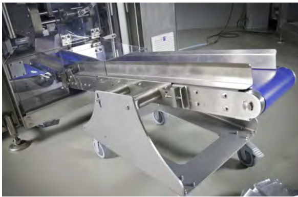
Conveyor with closed belt body
