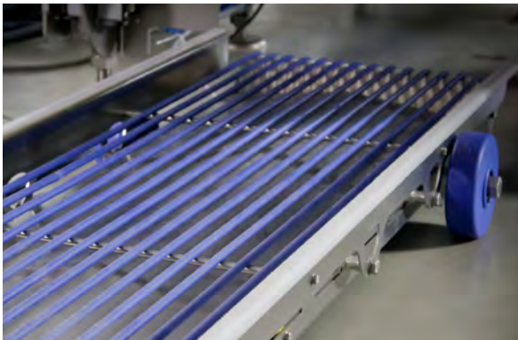
Conveyor with open body and individual belts
