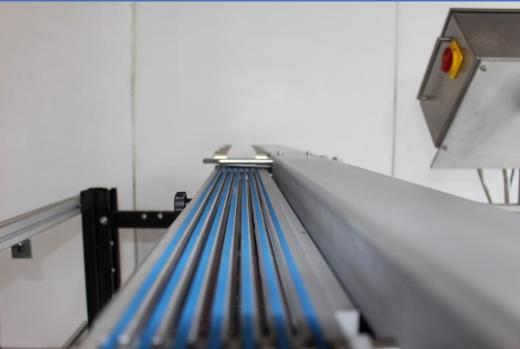
The CWL 150 Labeller is designed for high - speed labelling on to thermoforming machines for vacuum packing.
