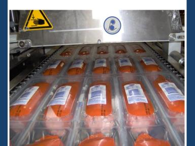
The CWL 150 – CrossWeb Top or Bottom Labeler is designed to easily mount on to your thermofirming packaging machine.
