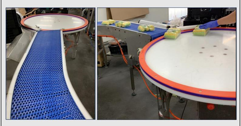
Our rotary accumulation turntable configurations can handle multiple containers sizes and products. The rotary design is flexible and the top discs diameters are 900 mm and 1200 mm.
