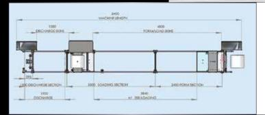
Machine Length: 8400 Discharge: 1500 mm Min. \* Forming/Loading: 3840 mm Max.
