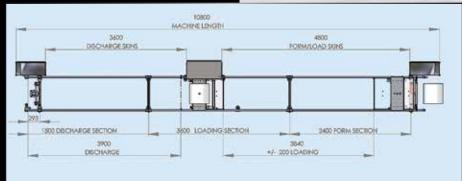
Machine Length: 10800 Discharge: 2400 mm Min. \* Forming/Loading: 4800 mm Max.
