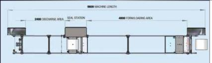
Machine Length: 9600 Discharge: 2400 mm Min. \* Forming/Loading: 4800 mm Max.
