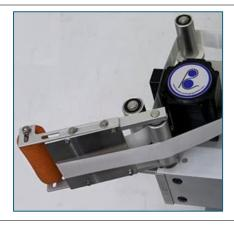
The label dispensing station is responsible for the precise application of the labels. After the labels have been detached from the backing strip, the backing strip is wound onto the backing paper rewind.
