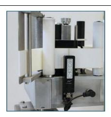
FC-4100 capacitive label Sensor suitable for paper and transparent labels. Quick teach button.
