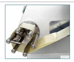
Guide the end of the backing strip through the coiler.
