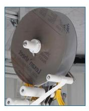
The unwinder receives the label tape. The flanged disks are secured with quick release buckles.
