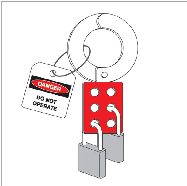
Figure 3 – Example of tag and lockout with the padlocks of two employees
