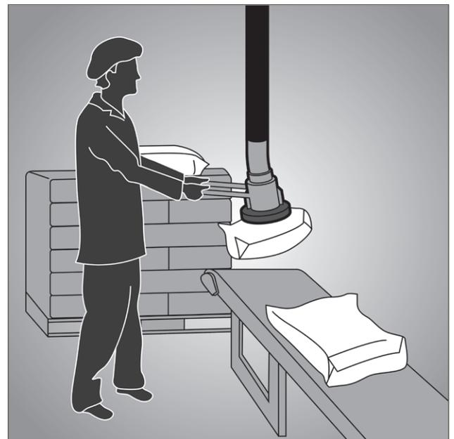
Figure 45 – A vacuum lifter reduces the need to bend and lift when palletising
