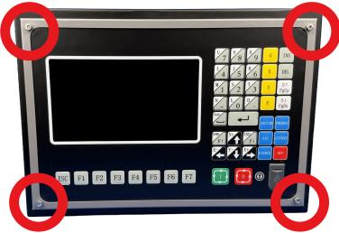
• Gently pull the operator station out from the shell and disconnect the cables with a Phillips Head screwdriver. Set the operator station aside.
