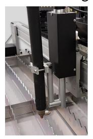
The mount that comes installed on the table designed for a hand torch. When installing a hand torch, be sure to place the torch head as deep into the mount as possible. Depending on the style of
