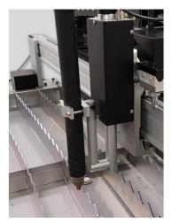
The mount that comes installed on the table is designed for a hand torch. When installing a hand torch, be sure to place the torch head as deep into the mount as possible. Depending on the style of torch, you
