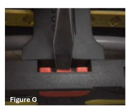
Take the flathead screwdriver and press the screwdriver's tip against the central red tab holding the track clip in place on one side (Figure G). Apply pressure to the red tab and the piece should slide out of the side of the chain (Figure H).
