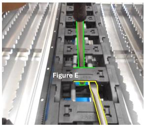
Using one screwdriver at the back of the clip, apply forward pressure, and pry up on the front of the clip with the second screwdriver. (Figure E).
