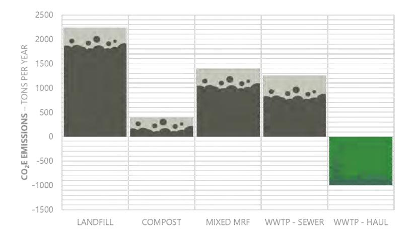
"From a carbon footprint comparison, the WWTP/Hauler alternative had the lowest carbon dioxide equivalent (CO<sub>2</sub>E) emissions compared to the other alternatives"
