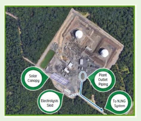
Electrolyzer will source solar power from a 416 kw DC array on site
