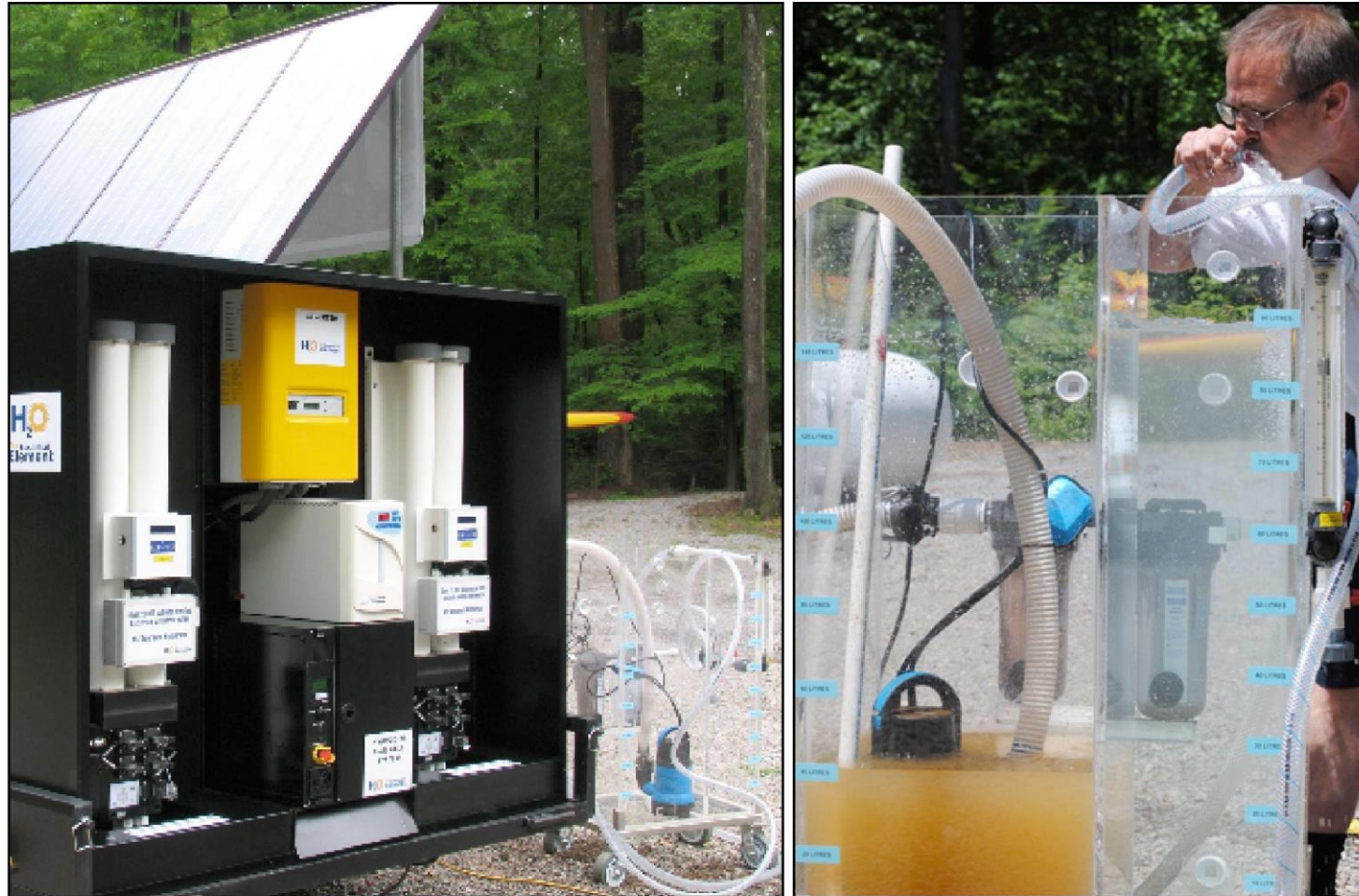
HYDRA H 2 O purification plant produces the highest quality water while the hydrogen generator splits water into hydrogen & oxygen; Co-Inventor & CTO Mike Strizki takes a drink of HYDRA purified water
