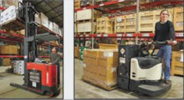
Class-1, -2, and -3 Forklifts Plug Power (GenDrive FCs)
