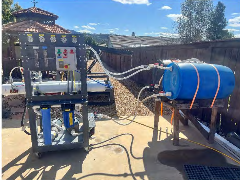
4.1.1.1 GVA-4000 Inlet and Outlet Water Connected
