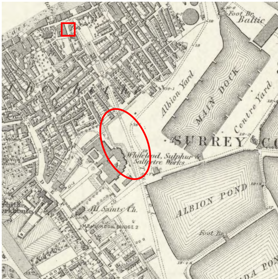
Figure 7 Essex Sheet LXXXI - surveyed 1862-1873 - published 1870-1882. In the red oval the embankment of tipping soil from the building of the docks nearby. It is also visible as dotted line the tunnel under the Thames of the East London Railway (currently use by the overground service). In the red square, the position of the current Brunel Museum, originally designed the shaft to access the tunnel. Meanwhile, from 1851, the names of the docks have changed: the three ponds of the Grand Surrey Dock are now identified as Main Dock, Albion Pond, Canada Pond.
