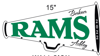
WALL SIGN MADE OF 1/4" PVC MOUNTING STRIPS ON BACK
