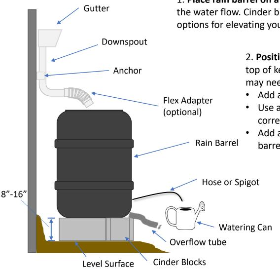
1. Place rain barrel on a flat, raised surface to allow gravity to help with the water flow. Cinder blocks or a wooden stand are simple, inexpensive options for elevating your rain barrel.
