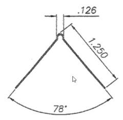
TOLERANCES: PROFILE ±1/16 ANGULAR ±3 Steel Profile: Steel Grade: Coating: ASTM C645 | ASTM A1003 | ASTM 653
