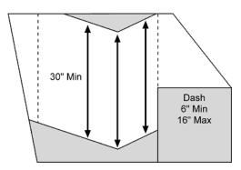
In the above example, the top trailing edge of the dash defines the vertical plane that is used to establish the front-to-back Free Space area. This example also depicts how changes to the roof build-down and floor build-up can be made provided a minimum al distance of 30 inches is maintained. Not to Scale.
