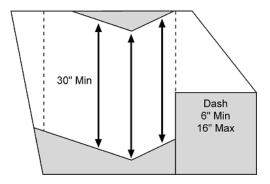
In the above example, the top trailing edge of the dash defines the vertical plane that is used to establish the front-to-back Free Space area. This example also depicts how changes to the roof build-down and floor build-up can be made provided a minimum al distance of 30 inches is maintained. Not to Scale.
