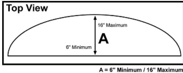
The plane of the dash bounded in the front by the firewall, in the back by the trailing edge of the dash, and for a distance of 12 inches to the left and 12 inches to the right (measured horizontally) of the sensor placement location must be completely flat with respect to the ground.
