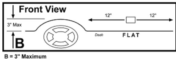
The dash may be completely solid (with no holes or perforations) and must extend front-to-back from the firewall to the trailing edge of the dash, and side-to-side from the windshield pillar on the driver's side to the windshield pillar on the passenger side.
