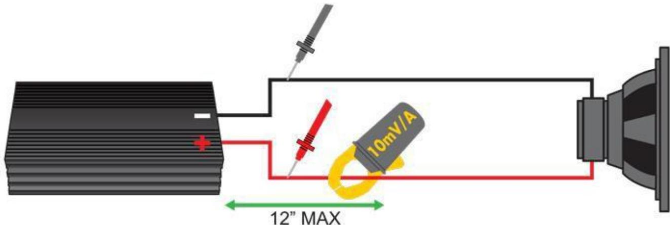
**Note 1:** The probes and clamp must be located within 12 inches of the speaker terminals on the amplifier.
