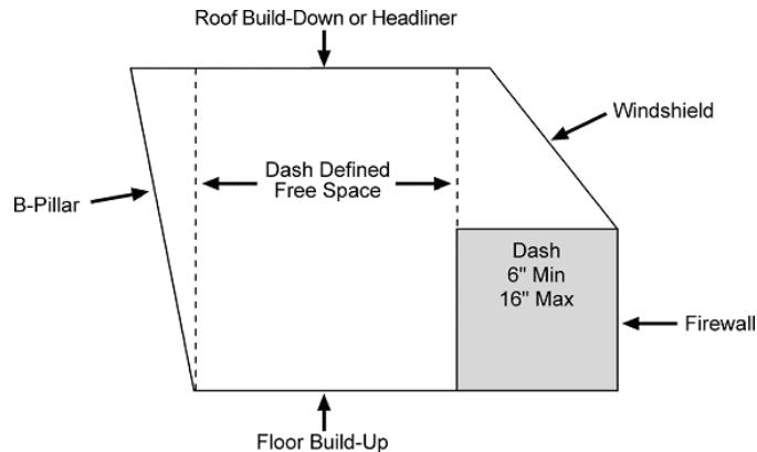
In the above example, the top trailing edge of the dash defines the vertical plane that is used to establish the front-to-back Free Space area. (Note how the dash is NOT located completely beneath the OEM windshield location.) Not to Scale.
