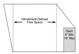
In the above example, the OEM top windshield frame defines the vertical plane that is used to establish the front-to-back Free Space area. (Note how the dash is located completely beneath the OEM windshield location.) Not to Scale.
