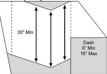
In the above example, the top trailing edge of the dash defines the vertical plane that is used to establish the front-to-back Free Space area. This example also depicts how changes to the roof build-down and floor build-up can be made provided a minimum all distance of 30 inches is maintained. Not to Scale.
