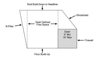
In the above example, the top trailing edge of the dash defines the vertical plane that is used to establish the front-to-back Free Space area. (Note how the dash is NOT located completely beneath the OEM windshield location.) Not to Scale.
