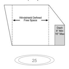
In the above example, the OEM top windshield frame defines the vertical plane that is used to establish the front-to-back Free Space area. (Note how the dash is located completely beneath the OEM windshield location.) Not to Scale.
