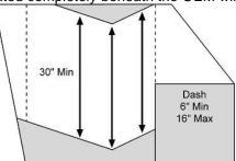
In the above example, the top trailing edge of the dash defines the vertical plane that is used to establish the front-to-back Free Space area. This example also depicts how changes to the roof build-down and floor build-up can be made provided a minimum all distance of 30 inches is maintained. Not to Scale.
