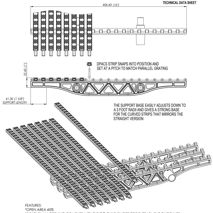
\*0.315" (8MM) OPENING COMPLIES WITH THE **IBC** CHILD FINGER/TOE ENTRAPMENT GUIDELINES \*CERTIFIED LOAD CLASSIFICATIONS UNDER **IBC** STANDARD AS 3996 CLASS "A" AS OVER 10kN FOR GRATES AND COVERS
