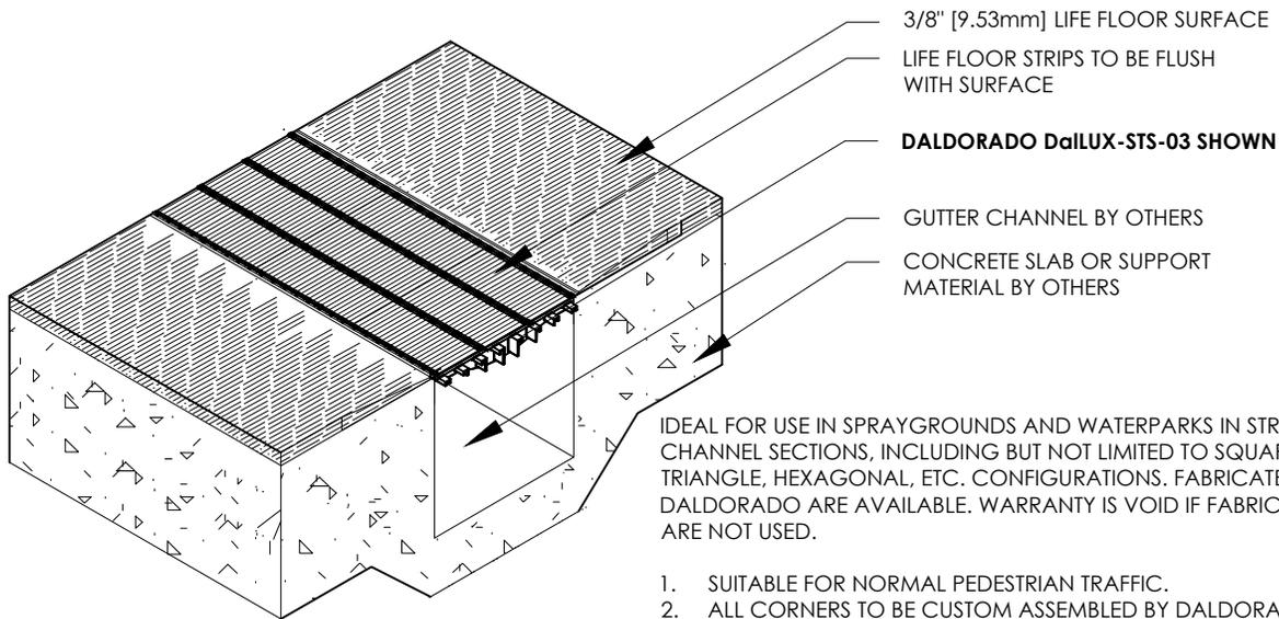
IDEAL FOR USE IN SPRAYGROUNDS AND WATERPARKS IN STRAIGHT GUTTER CHANNEL SECTIONS, INCLUDING BUT NOT LIMITED TO SQUARE, RECTANGULAR, TRIANGLE, HEXAGONAL, ETC. CONFIGURATIONS. FABRICATED CORNERS BY DALDORADO ARE AVAILABLE. WARRANTY IS VOID IF FABRICATED CORNERS ARE NOT USED.
