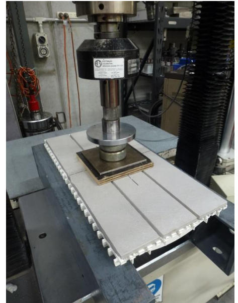
FIG. 2 GRATE TEST SET-UP
