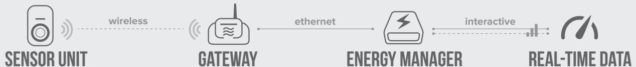
Enlighted Smart Sensors are connected to each light fixture in the building and collect occupancy, ambient light, temperature and energy consumption data. You can configure control profiles for different space types or occupant needs. Once configured, each sensor operates on its own without requiring centralized control.
