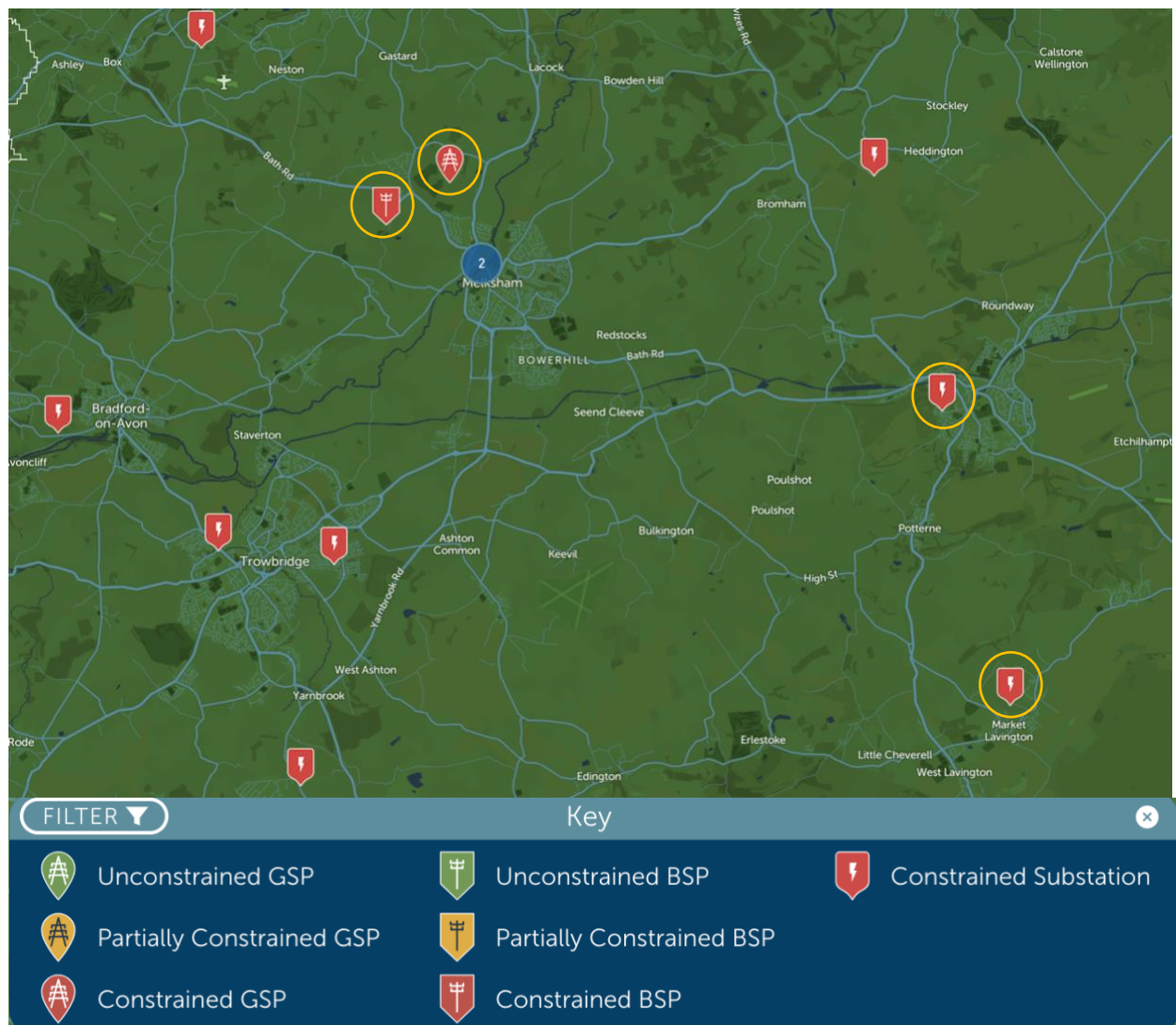
Fig 2. Capacity for Devices and surrounding area substations and their upstream BSP and GSP in Melksham - SSEN Generation availability heat map
