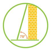
Angle ladders to minimise the risk of slipping outwards: as a rule of thumb this should be '1 out for every 4 up', (approximately 75°)
