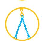
Lifting Accessory: Item used to attach load to lifting equipment e.g. chains, ropes, slings, etc.
