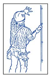
**ERECT** panels and fasten with Ultra-low Clip Screws. (Included with the Clips)
