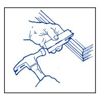
**INSERT** a few clips into each panel edge with the magnetic tool provided.
