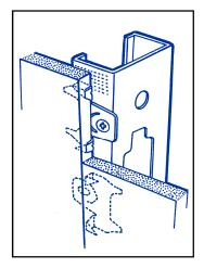
**SLIDE** the next panel clips behind for rock solid tongue & groove joints.
